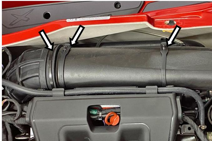
Loosen hose clamp securing OEM blow-off valve to rubber air intake hose. Loosen hose clamp securing rubber air intake hose to supercharger inlet.
