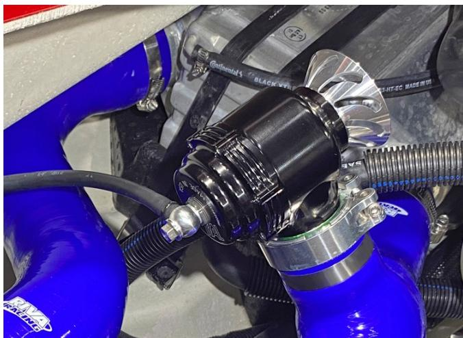
Orient vacuum hose fitting so that vacuum hose routes between blow-off valve and intake manifold fitting without becoming pinched. Secure banjo bolt. **NOTE: DO NOT overtighten banjo bolt.**
